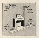
Cool air from floor level is heated in the double-walled Heatilator firebox, then returned to the room
