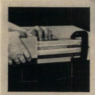
TO SAND THE END OF A BOARD without rounding the edges or breaking corners, clamp scrap lumber to both edges as shown.
