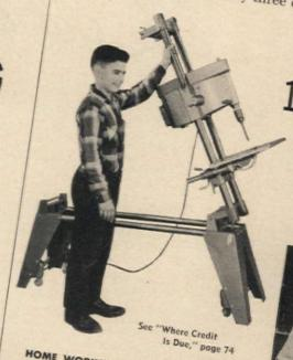
HOME WORKSHOP PROJECTS both large and small can call for operations requiring several tools. Here's a simplified, efficient power tool that with quick changeovers can easily handle a lot of jobs-sawing, dadoing, sanding, drilling, jigsawing, lathe turning. Unit includes 8" saw, 12" disc sander, 28" lathe, 16½" drill press and horizontal drill, for \$179.90. Bench (\$19.95) and ½-hp motor (\$34.95) are extra.
