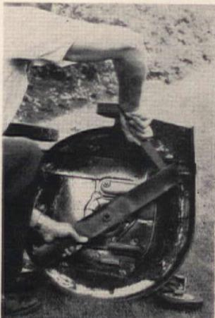
**EQUIPMENT CARE** . . . means better work and longer use from your lawn tools. And remember to handle all tools safely. Quick-sharpen a rotary mower with a file, but disengage the spark-plug cable before touching the blade.
