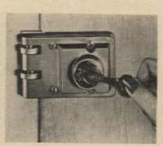
A worthwhile improvement over the traditional sash lock is the key-operated Win-Loc (photo, above left). It installs in the sash frame. Just drill a ½-inch hole and insert it. Installed in the center rail, it holds the window tightly sealed. In a side rail, it can hold the window either closed or partly open. Made by Win-Loc Corp., and offered at \$2 each.
