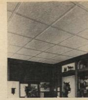
Someone's finally improved the stark, commercial appearance grid ceilings. Armstrong has introduced a 2 by 2 foot acoustical tile with beveled edges that hangs slightly below the supporting strips. The resulting shadow edge effect is accentuated by a gray tint on the bevels. A 12 by 16 foot Gridline Cushiontone ceiling, including necessary parts for the metal supporting grid, costs under \$80.
