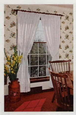
Windows can insulate elegantly. Colonial windows are more practical now, with PPG Twindow\* insulating glass. Twindow is two pieces of glass, with a slice of dry air sealed in between at the factory. Twindow looks like an ordinary window, but does extraordinary things—like providing many of the insulation benefits of a storm window. Reducing downdrafts. And keeping your home warmer to cut fuel bills. Twindow gives you colonial charm with modern convenience.
