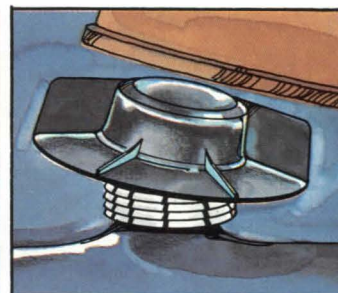
3 Snap and screw on threaded black cap.
