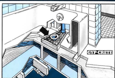
Opening under tub, shower drain and trap cavity must be caulked to prevent impact and conductive noise transmission.
