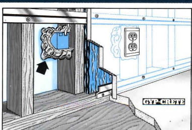
Outlets should be staggered in stud partitions and any opening in and around box sealed with caulking.
