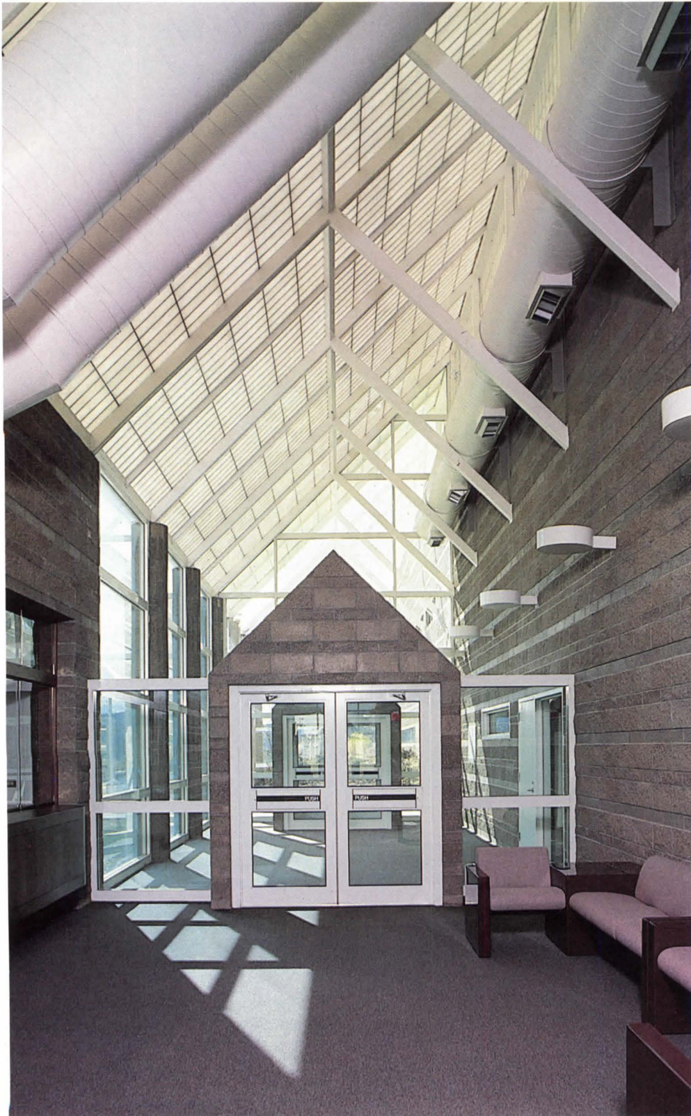
Above, interior lobby/corridor with translucent panels insulated to a .15 u-value providing daylighting and passive solar heating to the public spaces and courts. The environmental advantages of the glazing, however, outweigh its energy benefits, according to Muchow. Above right, the courtroom. Across page, a second view of the classical columns, this time at dusk, standing like Pretorian guards before the relentlessly modern, block and glass building.
