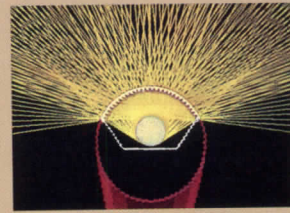
A selection of specially-designed lenses distributes light facet by facet. This up light combines wide spread with low lens brightness.
