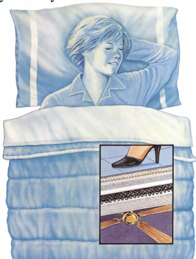
A floor that floats on Enkasonic matting protects the people below from the noise of those above. See Sweets 13081/BAS.
