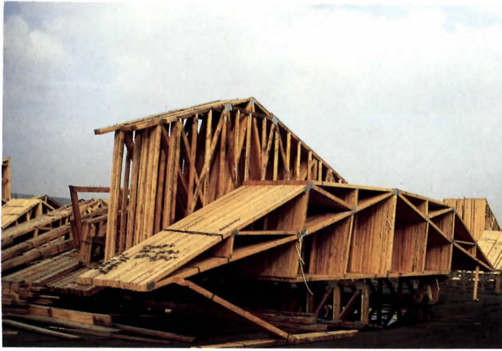
Above, mass-produced components including walls, trusses, and gable ends, stored and ready for shipment. Right, interior of U.S. component manufacturer's housing factory.
