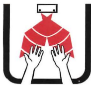
The ACCU-ZONE advantage—two zone-focused infrared transmitting beams create a large detection zone confined strictly to the bowl.
