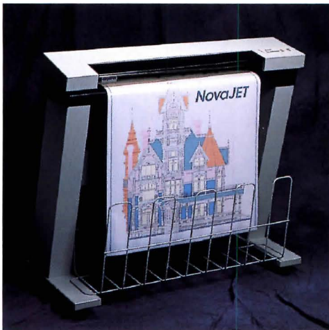
Enter Computer's new NovaJet 300 DPI color inkjet plotter (above) produces 256 colors at up to E size.
