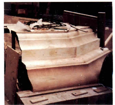
CORNICE MOLD: Built of wood.
