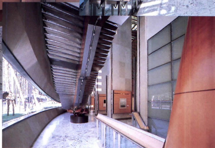
Grand staircase is cantilevered from single, continuous concrete beam, and leads to upper gallery and retail banking offices (left). Carpenter-designed glass wall, supported by aluminum and stainless steel armature, changes color of room throughout the day.
