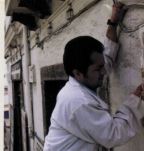
In Quito, Ecuador, conservator takes paint samples to determine original color of commercial building.
