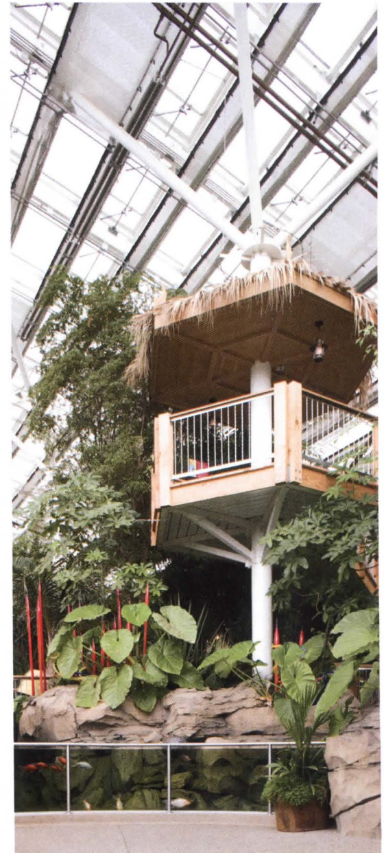
Plant beds (above) have root-zone heating, so the canopies of the plants can endure cooler temperatures without suffering. Mistlers deliver a fine spray of water to plant canopies as needed, and in summer ultrasonic foggers near the footpaths introduce evaporative cooling locally. Radiant heating in the footpaths provides supplementary heat when needed.
