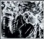
Xypex Crystallization (Initiated)
