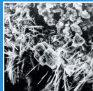
Xypex Crystallization (Initiated)
