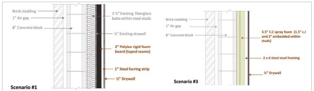
The two retrofit scenarios, down-selected for field demonstration through this project, were installed in two of the eight zones in the FRP.
