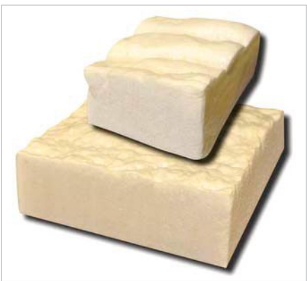
Closed-cell (ccSPF) and open-cell (ocSPF) Spray Polyurethane Foams serve as effective air barriers and insulation but have different properties.
