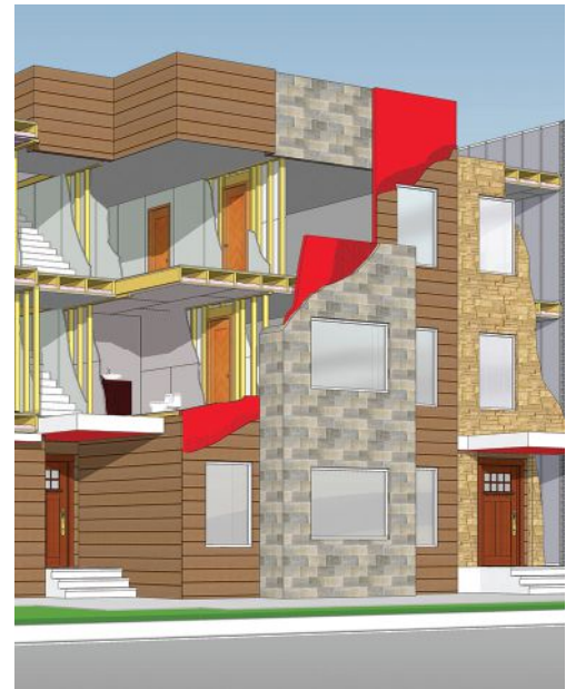
Shown in red, exterior sheathing gypsum panels are an ideal underlayment for a wide range of exterior wall cladding materials typically specified for multi-family projects; they are designed to help the wall assembly resist air and water infiltration, mold growth, noise transmission and flame spread.
