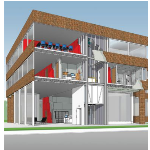
Shown in red, abuse-resistant gypsum panels provide a tougher, more durable version of traditional drywall to minimize cosmetic maintenance costs and repairs to walls in high traffic areas due to surface scuffs, abrasions and indentations.
