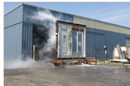
Fire-rated glass products with fire-ratings over 20 minutes must pass the required hose stream test.
