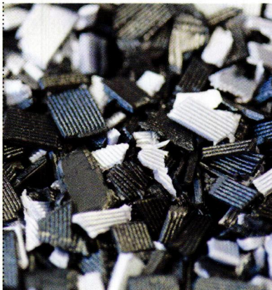
Shredded material from Signify's 3D-printed luminaires, which are recyclable
