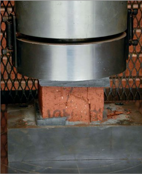
Capped brick specimen in compression test. Photo courtesy of The Bishop Materials Laboratory and the National Brick Research Center, Anderson, SC.
