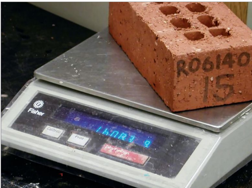
Weighing brick specimen. Photo courtesy of The Bishop Materials Laboratory and the National Brick Research Center, Anderson, SC.
