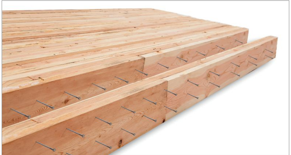
NLT is made from dimension lumber stacked on edge and fastened together with nails (or less commonly screws) to form a solid structural element. Photo courtesy of Think Wood.
