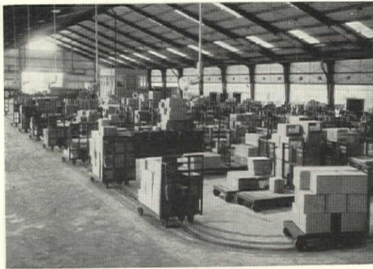
Interior of dock building showing drag line
