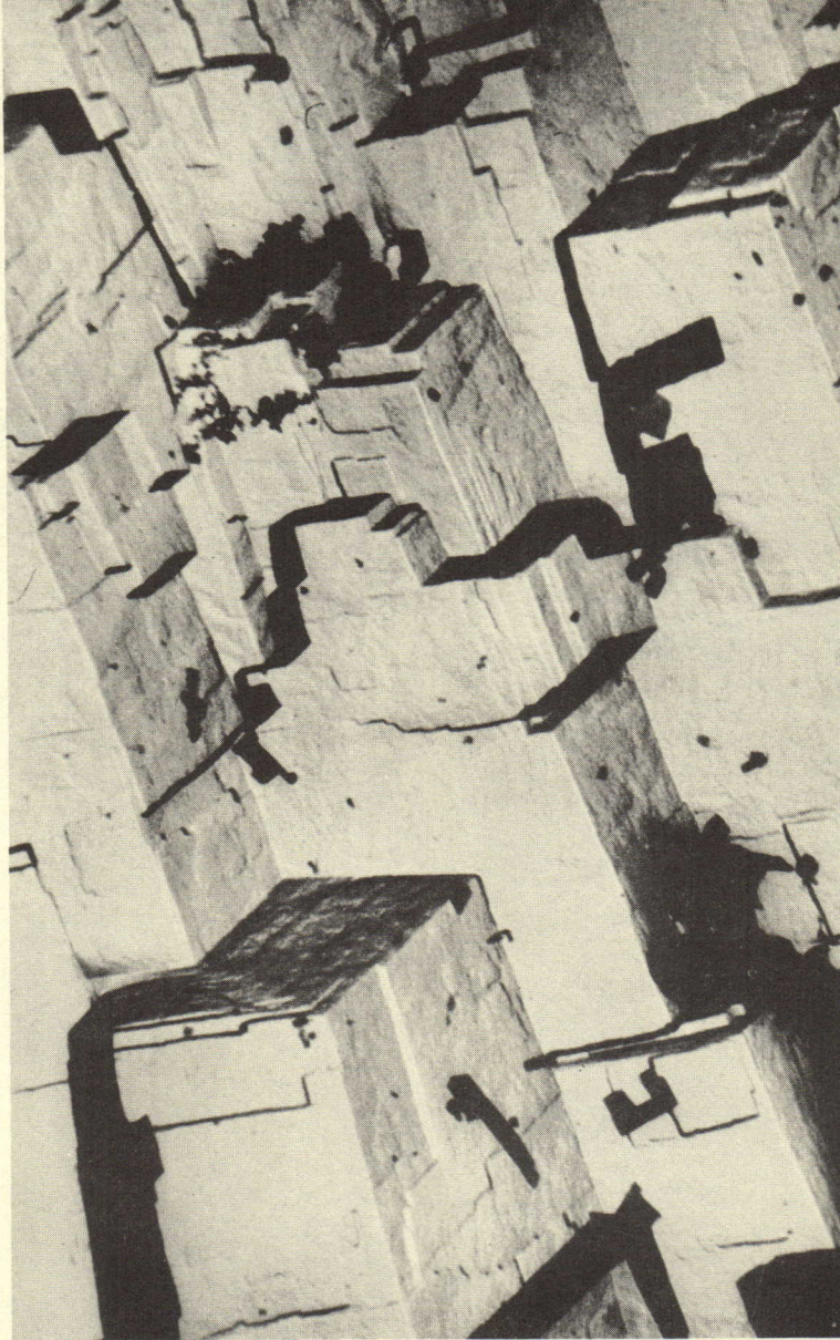
Surface structure of aluminum electronmicrograph 39,000:1. Photo: Dr Wegmann, Zurich
