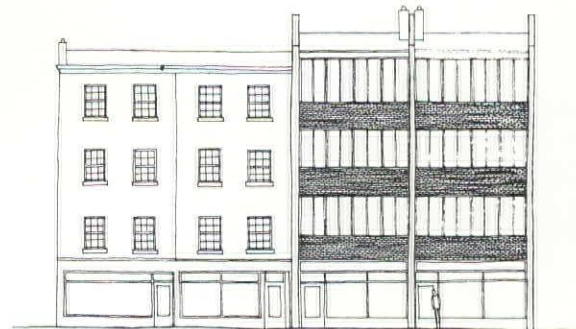
3 New building (Type A, illustrations 1, 2, 3) provides studio and living-space for artists. Large window areas face rear courts. Free-standing stair towers serve two or more buildings. Towers are glassed in for maximum natural light. Plan gives more space in main structure
