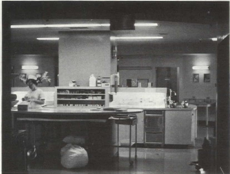
Nurses' station in center of circular nursing unit allows visual control, shorter walking distances to patient rooms
