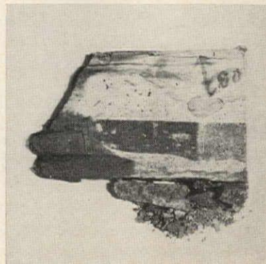
Second stage: edge of clay-rich dolomite crumbles under same action.
