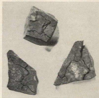
First stage: wetting-drying action has caused dolomite rocks to crack.
