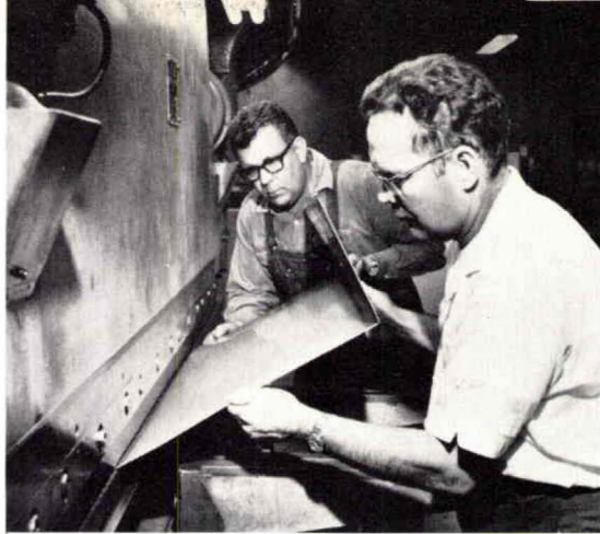
Pre-forming JalTEX stainless steel sheets at the Temp-Control Corp. plant. Edges for joining were crimped one-half inch for flat-seam joining.
