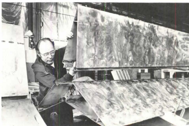
The assembly of 'Ad Astra' begins with the welding of triangular braces to one of three points to form the inner structure (top). Then center braces are attached to the first assembled point. Welder's sparks fly as a section of base plate is attached to a point of the sculpture. Next, one-third of a lower section is complete. Now the parts are joined to form a three-pointed star. The sculpture is near completion (bottom) before final assembly (above) at the site in Washington, D.C.
