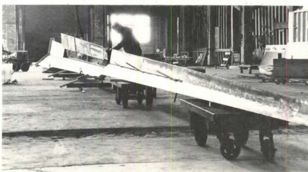
The assembly of 'Ad Astra' begins with the welding of triangular braces to one of three points to form the inner structure (top). Then center braces are attached to the first assembled point. Welder's sparks fly as a section of base plate is attached to a point of the sculpture. Next, one-third of a lower section is complete. Now the parts are joined to form a three-pointed star. The sculpture is near completion (bottom) before final assembly (above) at the site in Washington, D.C.
