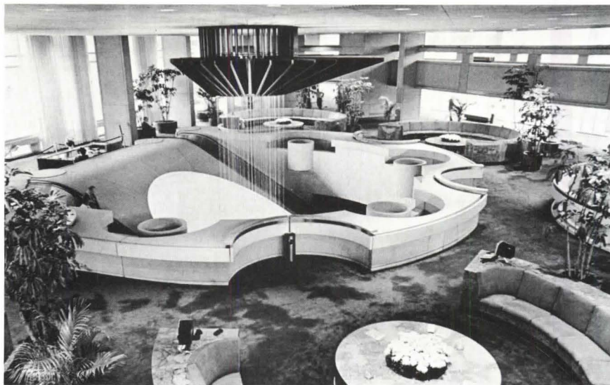
Display fountain in visitors' lobby aids humidity control in heating season.
