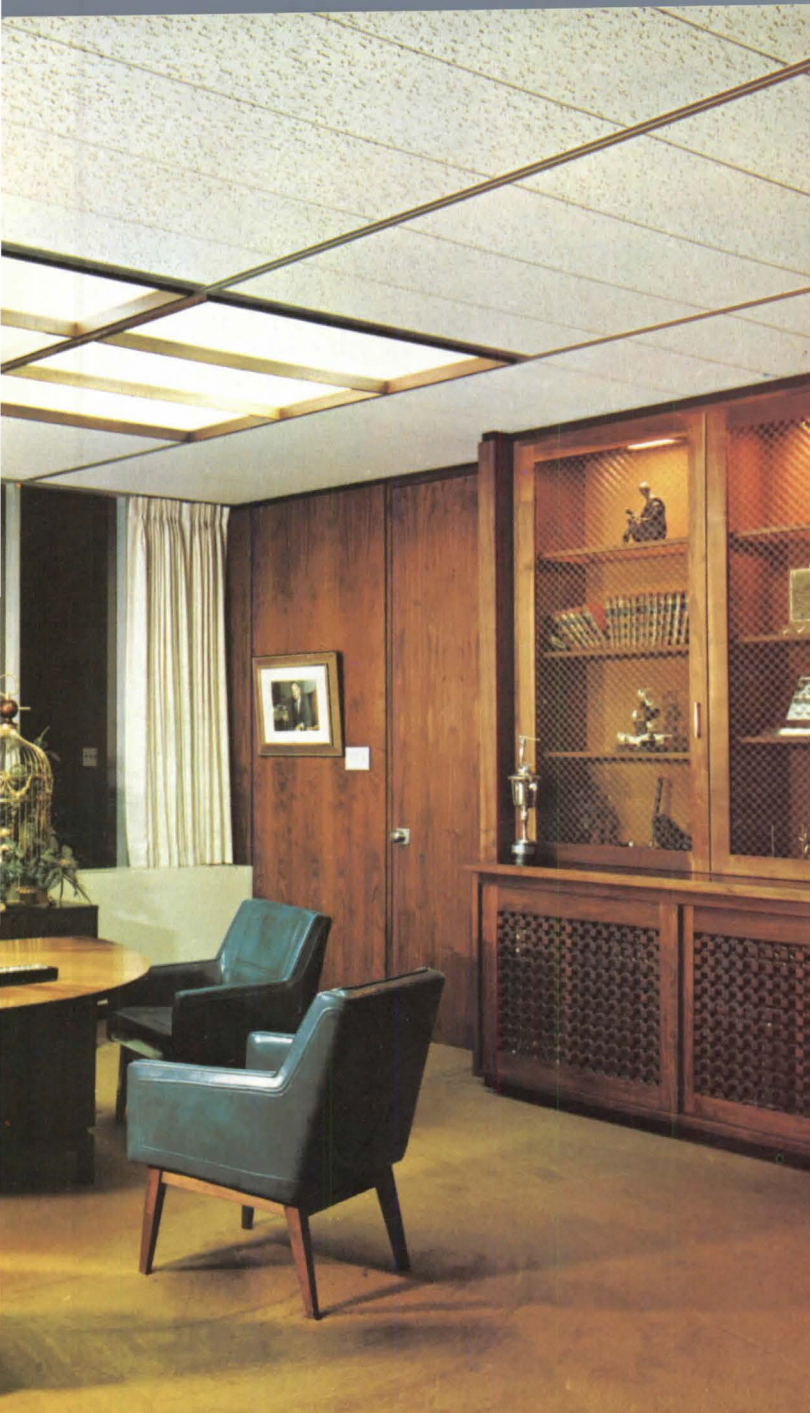
Solitude Tile (5/8" x 12" x 12") is beveled, kerfed and rabbeted . . . designed for installation with a concealed spline suspension system, or with adhesive.
