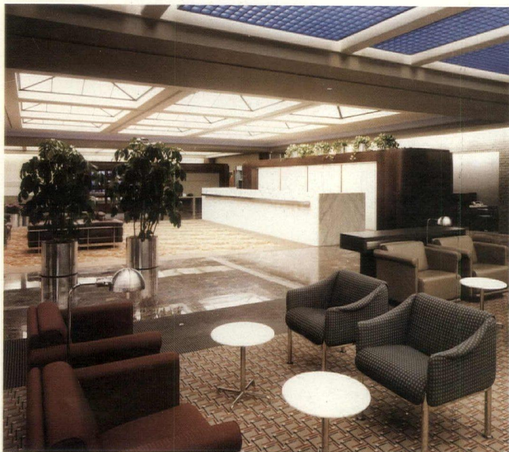
Blue walls washed with 2800K neon flank the escalators that take guests from the security check-in desk to club reception area. 3000K triphosphor fluorescent lamps in indirect fixtures are hidden in the ceiling lattice.
