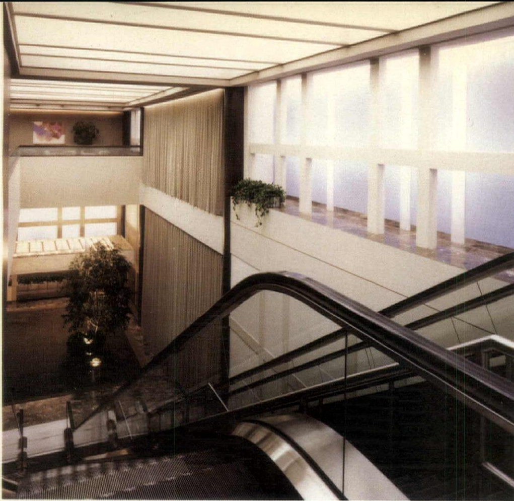
Blue walls washed with 2800K neon flank the escalators that take guests from the security check-in desk to club reception area. 3000K triphosphor fluorescent lamps in indirect fixtures are hidden in the ceiling lattice.
