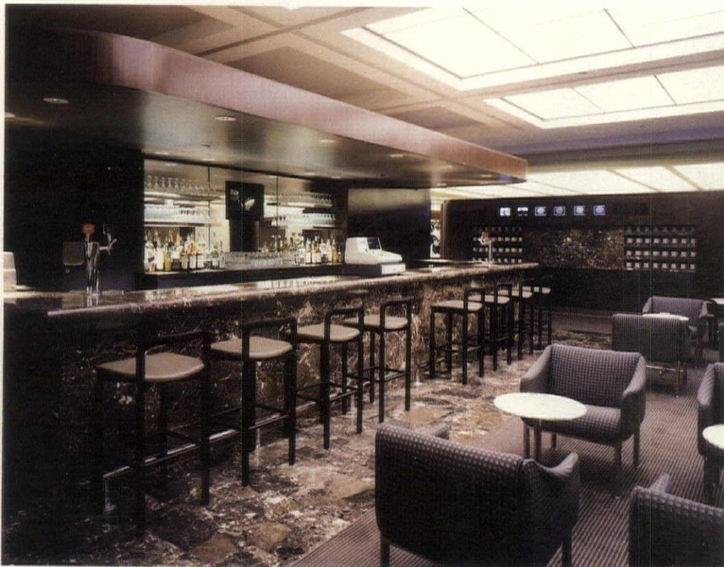
The bar is lit with flat acrylic panels backlit with 15-millimeter, 2800K neon that provide a soft, very warm glow. Low-voltage downlights highlight the bar, and fluorescent slots in the back bar highlight glassware.
