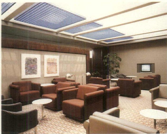
In lounge areas, spaces are further defined by blue grids suspended between beams carrying indirect fluorescent uplights, similar to those in the entry space. Incandescent floor lamps for reading and writing provide a further personal touch.
