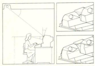
Figure 1: (Left) VDT workstation elevation, (top right) standard parabolic, (bottom right) compound parabolic.
