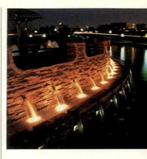
and two levels of cascading waterfalls that return the water to Little Dry Creek. The spouts of water empty into the mid-level, and the falls and masonry are highlighted from below by 250-watt incandescent PAR lamps. The lower waterfalls are lit from behind by 13-watt PL fluorescent lamps.
