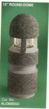
**DURABLE LIGHTING** - Dome Top Bollards constructed of reinforced precast concrete with a cast aluminum grill and an inner high impact acrylic diffuser encloses a variety of H.I.D. lighting. Choose from (3) standard mounting heights and (2) textured finishes. Concrete colors and ceramic tiles are available.
