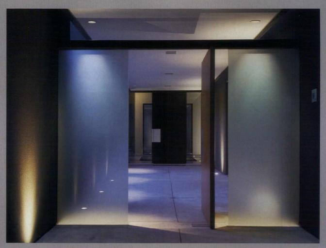
The MR16s perform different jobs: with a frosted lens, they act as downlights; with a soft focus lens, as art lights; and with no lens, as dynamic accent lights. The fixtures are aligned in a grid that accentuates the longitudinal axis of the house, drawing the eye from the living room through the dining room to the kitchen beyond.
