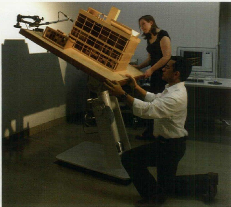
Physical modeling tools, such as a helidon—a tilt-table where a model is placed and a light source applied—enable designers to see how light moves through a space.
