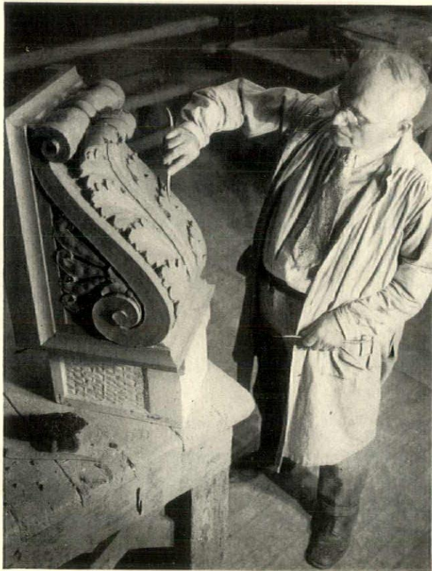
In the modelling studio. Here all ornamental details that depart from plain surfaces are modelled by sculptors or skilled modellers, to be approved by the architect before moulding
