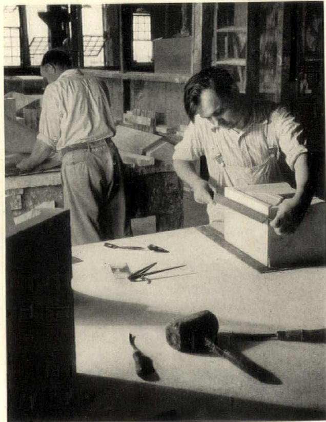
In the moulding shop. From the original models plaster moulds are here made. From these moulds an almost unlimited number of terra-cotta units can be manufactured, if desired
