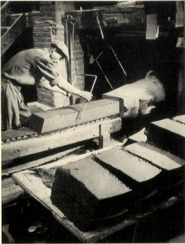
Clay milling again, where the clay is extruded and carried away on an endless belt. A workman cuts the continuous band of extruded clay into pieces that can be handled more easily
