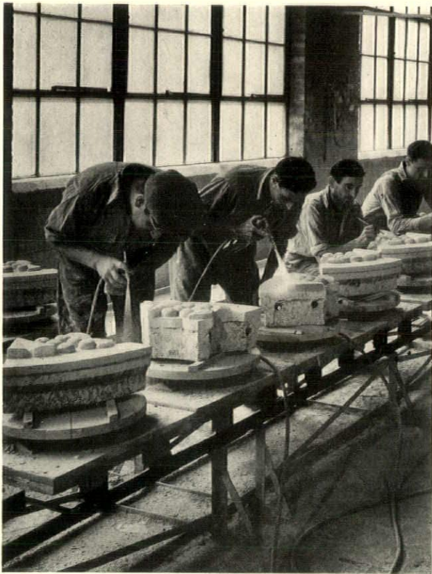
In the polychrome department, where the colors are applied by hand brush or air brush directly to the clay surface. Abbochrome colors are a mottled combination of three or more tones applied simultaneously
