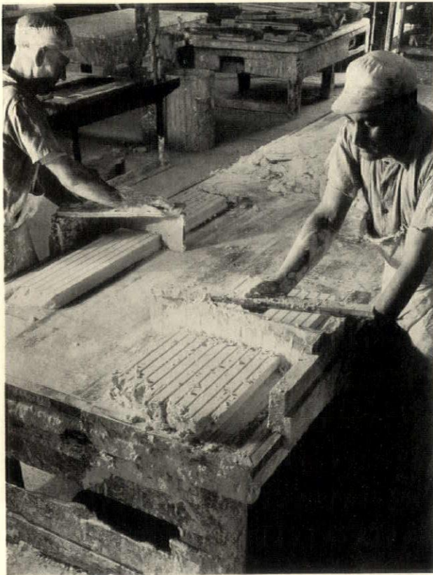
In the model-making shop. Plain units such as ashlar blocks or simple cornice details can be profiled in plaster of Paris. Small ornaments, as rosettes, modelled in clay, can be attached to the plaster model
