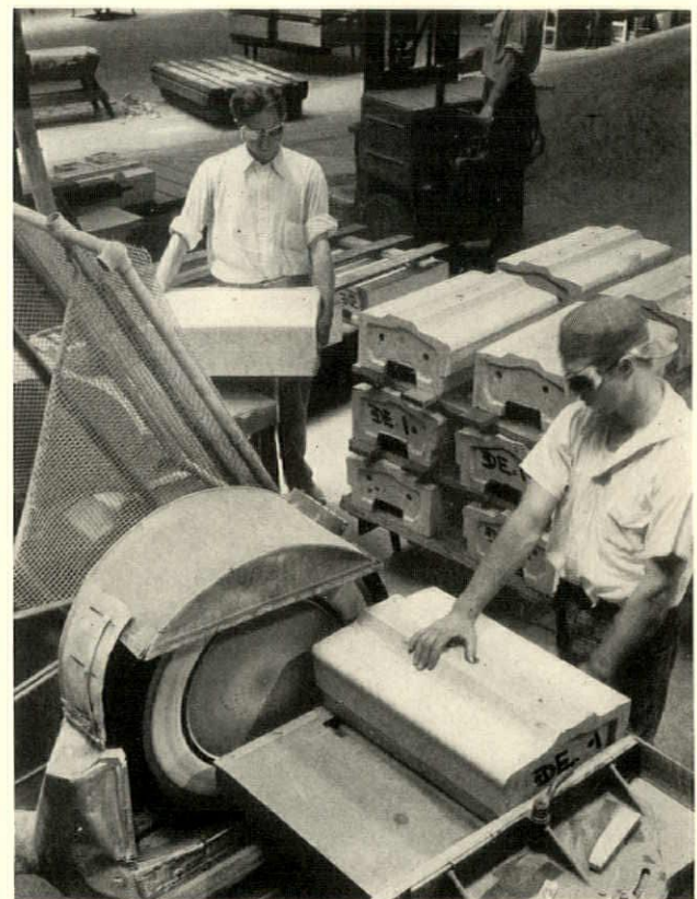
After firing, the terra-cotta is temporarily assembled, the joints being squared and cut to proper alignment or size. Here each piece is numbered to denote its position in the building
