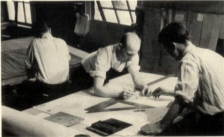
Making shop drawings of full-size details as derived from the architect's drawings. All full sizes, of course, are measured with a terra-cotta shrinkage scale—13 inches equal 1 foot
