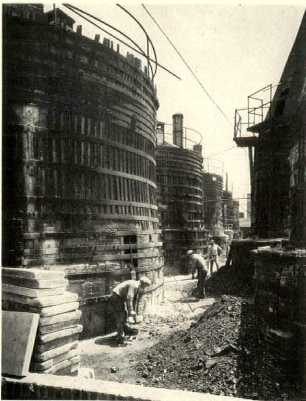
Firing the kiln. The heat is gradually increased until the temperature reaches 2300° F. Then the fires are dropped and the kilns are allowed to cool, causing a slow annealing of the terra-cotta
