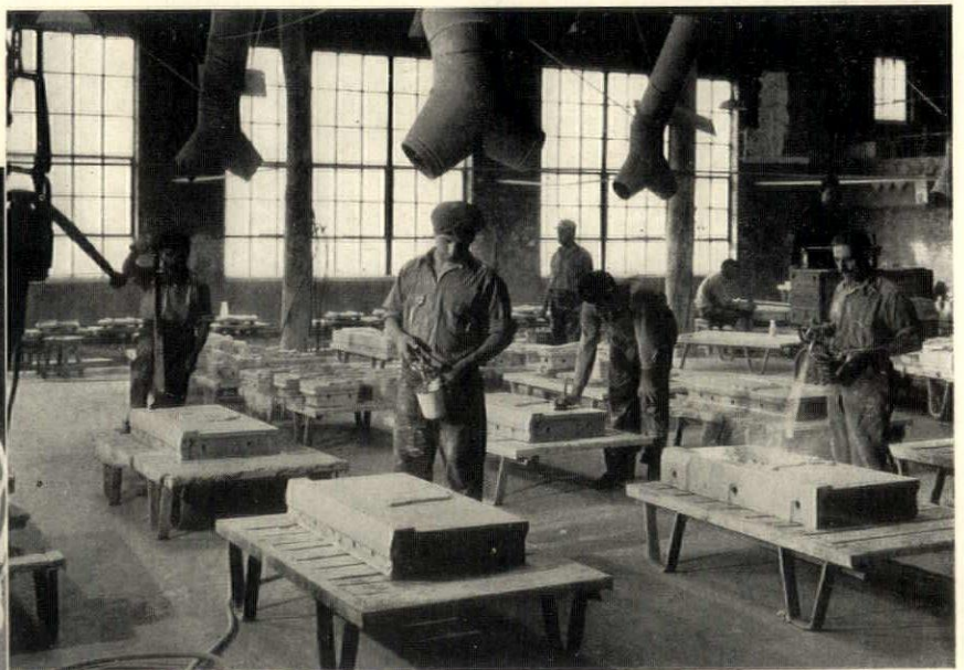
In the spraying department where, by means of compressed air, the exposed surfaces of the terra-cotta are covered with the ceramic mixture or "slip" which, in the firing, develops the desired color or glaze
