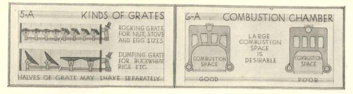
make sure that he specifies a large enough grate area. An oversized grate area allows a slower burning of gases and a consequently longer time for the heat units to be transferred to the water.
