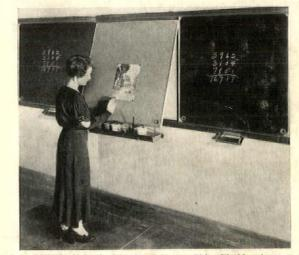
The New AUSTRAL Multi-Use Blackboard Fixture. Either Blackboard area or, when reversed. Corkboard area are available. Two metal brackets attached to the chalk rail strip permit the leaf to be brought forward into the easel position as shown above. The leaf may be removed entirely and serve as a display board
