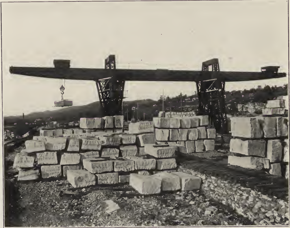
ONE OF THE GREAT CRANES FOR LOADING BLOCKS ON TO THE TRAINS.
