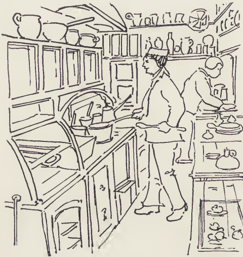
Kitchen in a private car. The bright iron range and broiler have hoods over to collect and disperse odors; the row of windows is seen over. The stove lids are depressed, so that nothing can slide off when the train is in motion.
