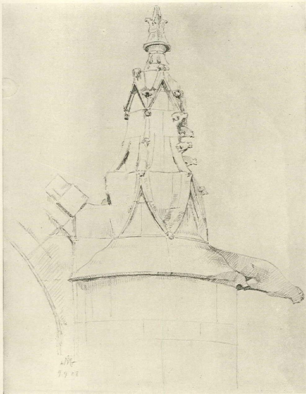
FIG. 168. TERMINAL OF STAIRCASE TURRET, ST. ETIENNE, BEAUVAIS. (Acting as respond to flying buttress.)
