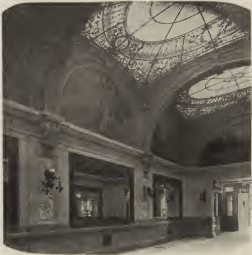
FIG. 8. HANGING FIXTURES HERE WOULD BE INCONGRUOUS. OPAQUE REFLECTORS ABOVE CEILING LIGHTS WOULD BE SUITABLE AND EFFECTIVE.
