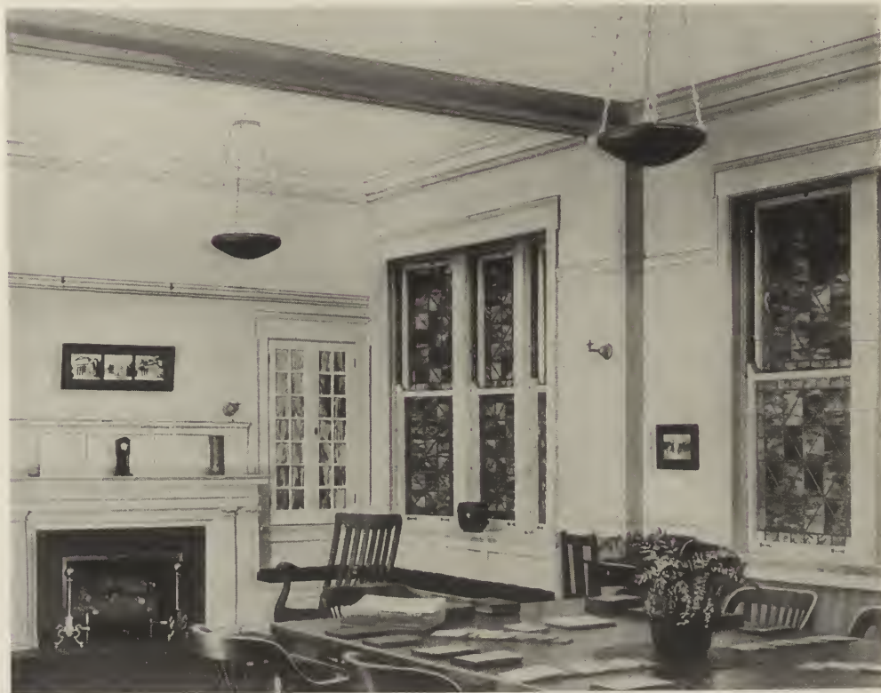
FIG. 1. THE AMOUNT OF USEFUL LIGHT REDIRECTED BY THE SIDEWALLS IS NEGLIGIBLE. GENERAL ILLUMINATION ON LIGHT COLORED WALLS, UNLESS RELIEVED BY DECORATION, IS PRODUCTIVE OF MONOTONY AND OCULAR FATIGUE.
