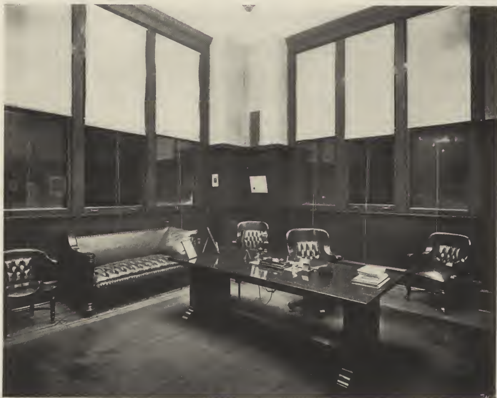
FIG. 2. A MODERATELY DARK WALL SUGGESTS PERSPECTIVE, AND BY CONTRAST WITH BRIGHT WORKING SURFACES, RELIEVES THE EYE. POLISHED TABLE-TOPS REFLECT EVERYTHING, ESPECIALLY GLARING LIGHT SOURCES PLACED ABOVE THEM.
