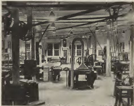
FIG. 9. INDUSTRIAL LIGHTING, WHERE GOOD GENERAL ILLUMINATION IS OBTAINED ECONOMICALLY BY OPAQUE REFLECTORS EVENLY SPACED, BUT NOT HUNG DIRECTLY ABOVE THE POLISHED SURFACES OF MACHINES.
