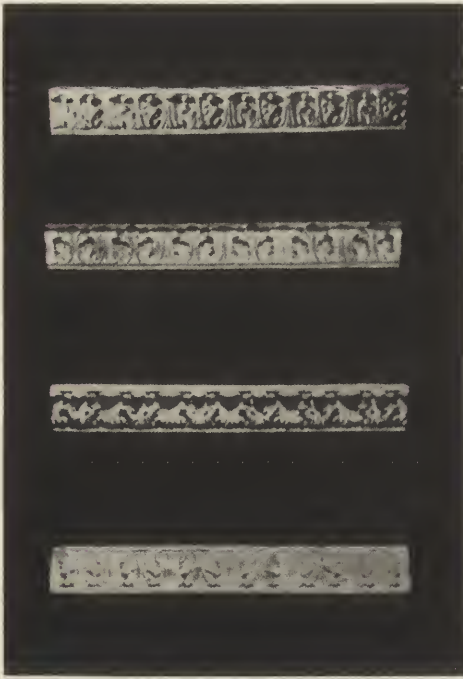
FIG. 4. VARIATIONS PRODUCED BY LIGHT FROM DIFFERENT DIRECTIONS ON BAS-RELIEF WORK. UNIFORM LIGHT FROM ALL DIRECTIONS OBLITERATES DETAIL.
