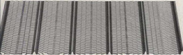
Ribplex plates are 24 inches wide and from 6 to 12 feet long—in gauges 24, 26 and 28. The ribs are \frac{3}{4} of an inch high and spaced 4.8 inches from center to center. Sample and further information on request.
