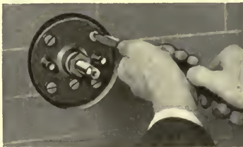
DIAL REMOVED. THE ONLY TOOL REQUIRED TO TAKE THE MIXER APART IS A SCREW DRIVER.
