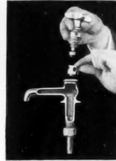
K-8067 Kohler Interchangeable Lavatory Faucet with compression unit. To change to self-closing type, take out removable seat and compression unit.
