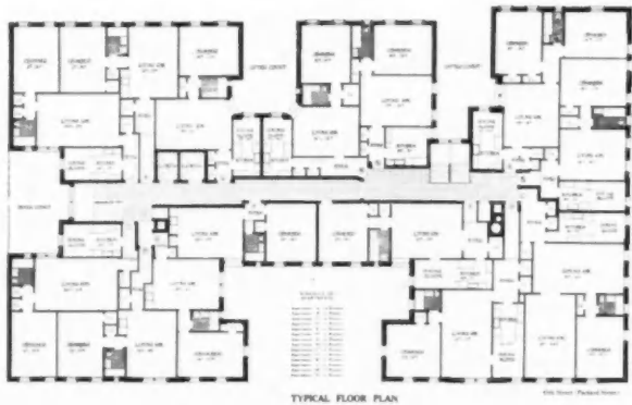
FIG. 12. "BUILDERS' APARTMENT." Example of 70 per cent coverage with wasteful corridor and foyers.
