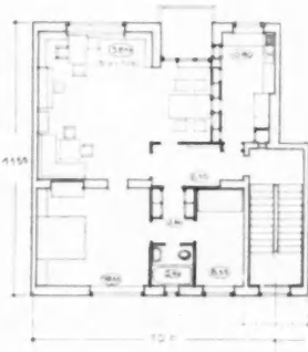
Fig. (e) Designer's study of a ground floor plan of same dimensions as Fig. (d). Staircase moved to avoid through-passage on ground floor
