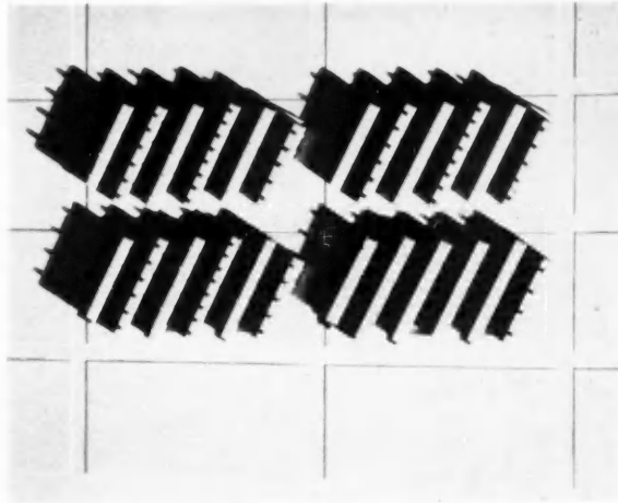
4. Shadows at winter solstice, Dec. 21, 9:00 A.M., C.S.T. Position of sun: 12° altitude, 50° S. of east point.
