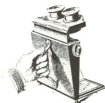
1890. Portable Stereopticon for prints; also in use was the Wheatstone tele-stereopticon for viewing nature directly through an arrangement of mirrors and prisms.
