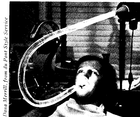
"Bent light". Some plastics have the property of internal reflection of light.
